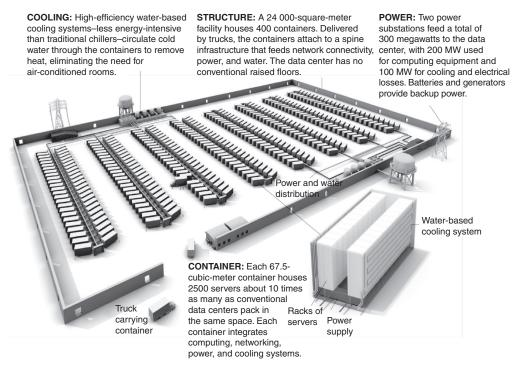
Figure 2.2 Expandable, modular cloud data center. Notice there is no roof. New containers with servers, power, cooling and network taps can be swapped in and out as needed. Source: *IEEE Spectrum* magazine.
